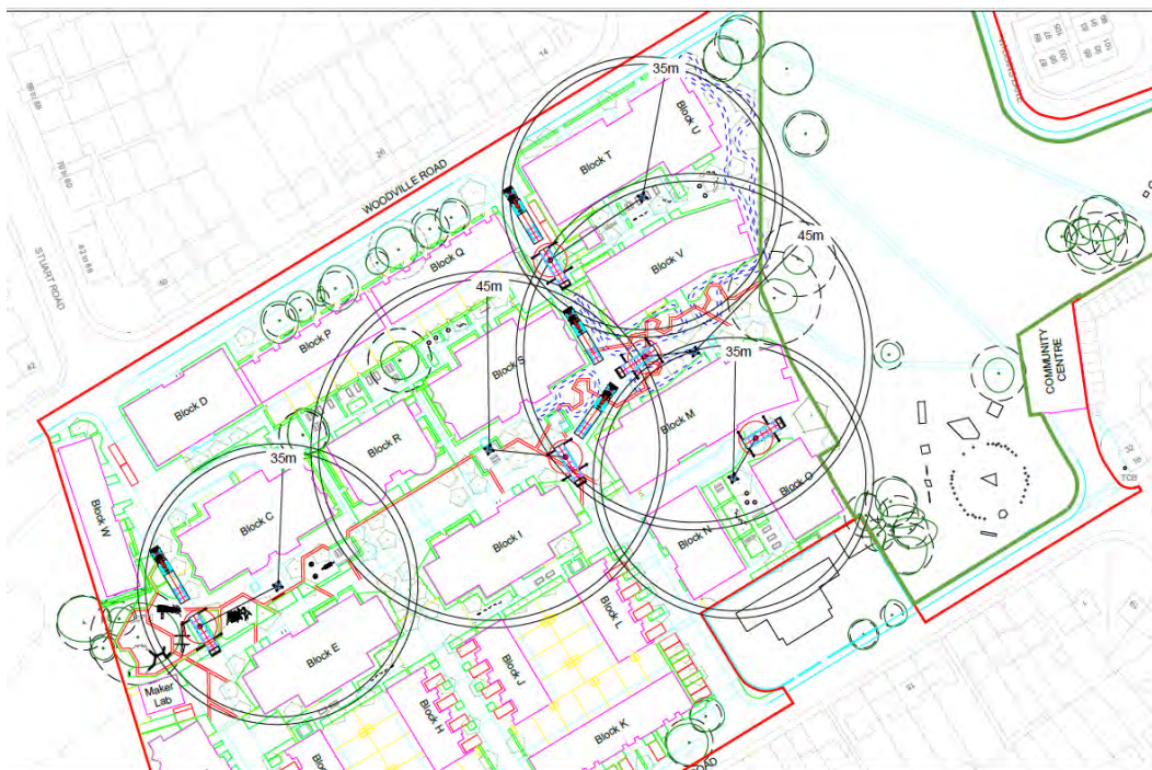
Figure 6 – Indicative Crane Positions
